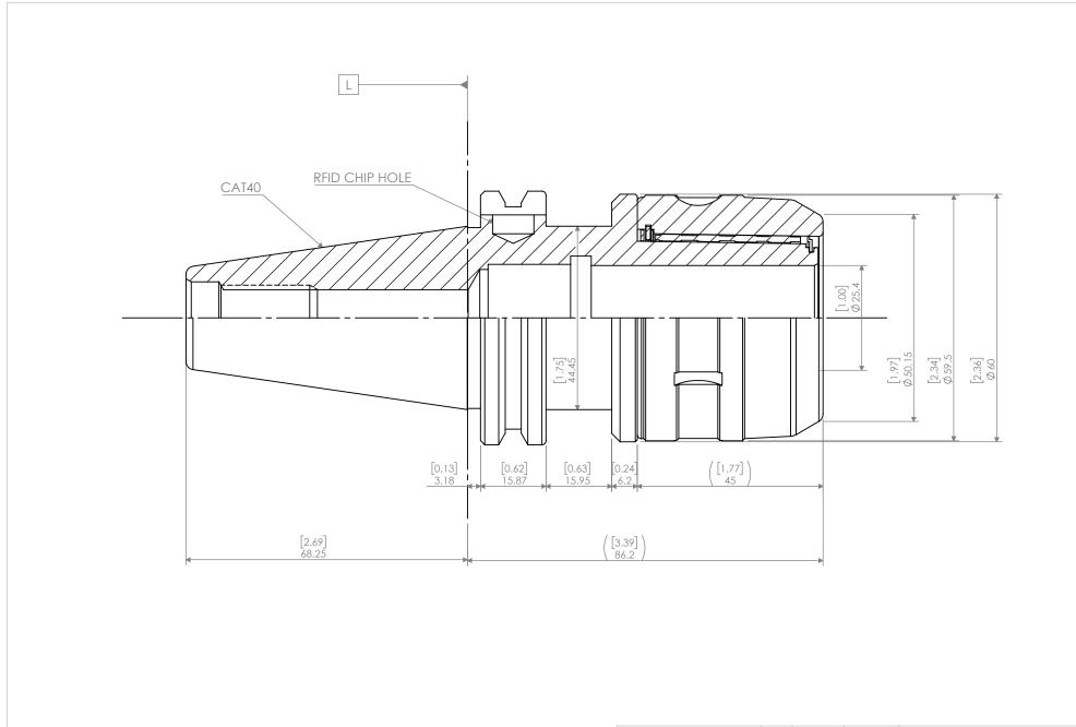
DATE CAT40 1" MILLING CHUCK IDCHIPHOLE NAME PROPRIETARY AND CONFIDENTIAL DRAWN BT 7/14/2021 THE INFORMATION CONTAINED IN THIS DRAWING IS THE SOLE PROPERTY OF LYNDEX NIKKEN. ANY REPRODUCTION IN PART OR AS A WHOLE WITHOUT THE WRITTEN PERMISSION OF LYNDEX NIKKEN IS PROHIBITED. DRAWING SUBJECT TO CHANGE WITHOUT NOTICE. NOTES: NIKKEN SIZE DWG. NO. REV. Α CAT40-C1-85U-IDU SCALE 1:1 SHEET 1 OF 1
